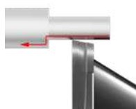
Small axial relief - stronger tool
