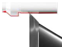
Large axial relief - weaker tool
