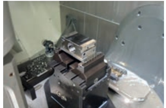
Grip and replace blank parts directly using the active gripper and clamping device.
