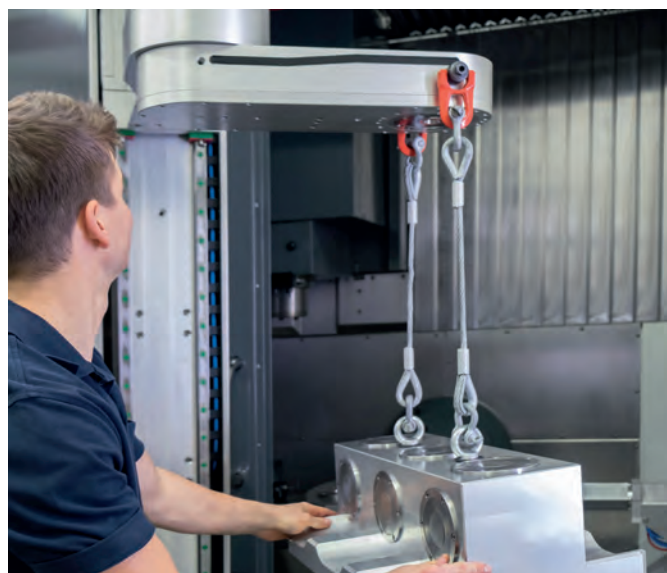
The robot can be used as a crane during manual operation due to its high load capacity.
