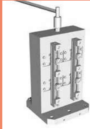
Multi-Rail RM units + hydraulics. Live system in horizontal machining center.
