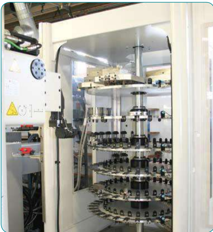
Magazine for palletising magnetic chucks and tools
