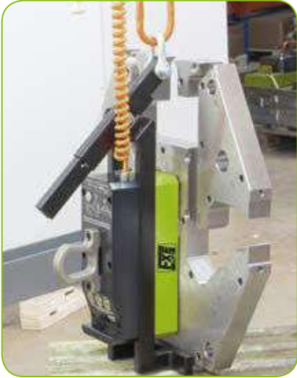
FXE HV device for horizontal/vertical lifting
