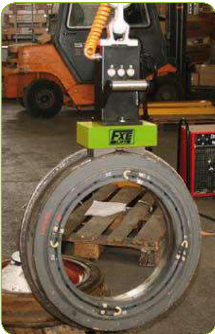
FXE with pole shoe for railway wheels
