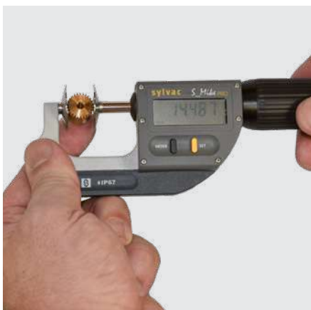
Part measurement with a S_Mike PRO Disk
