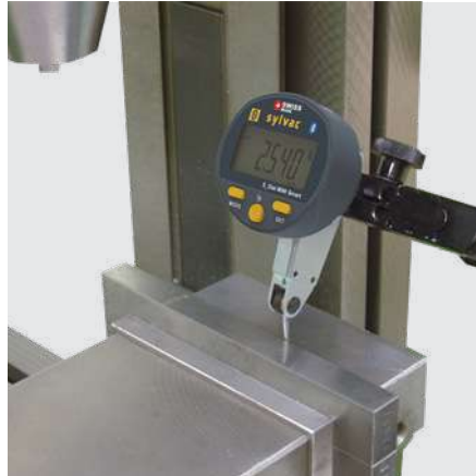
Checking the alignment on milling machine.
